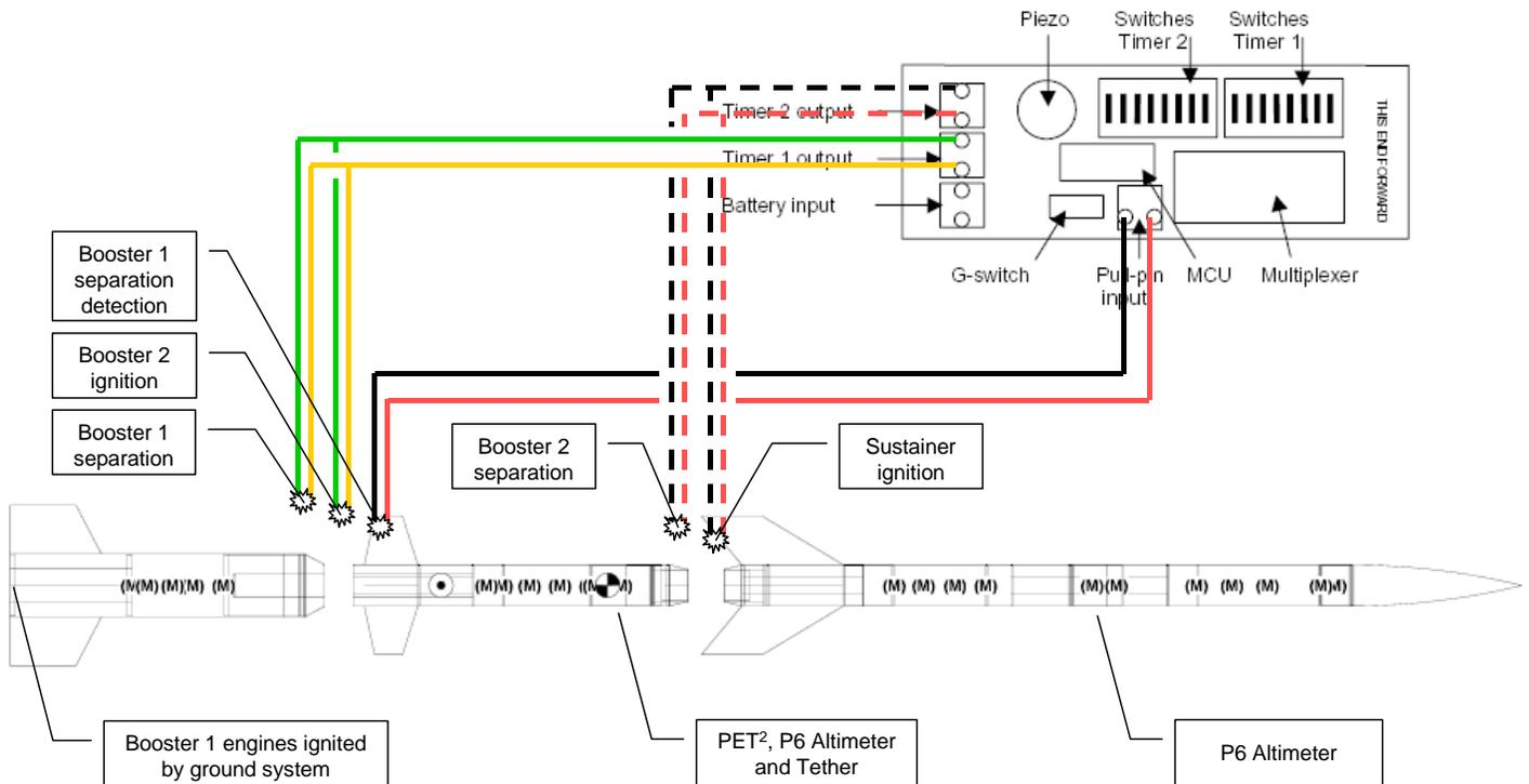
Here is how the design was intended to work and the planned flight profile.
